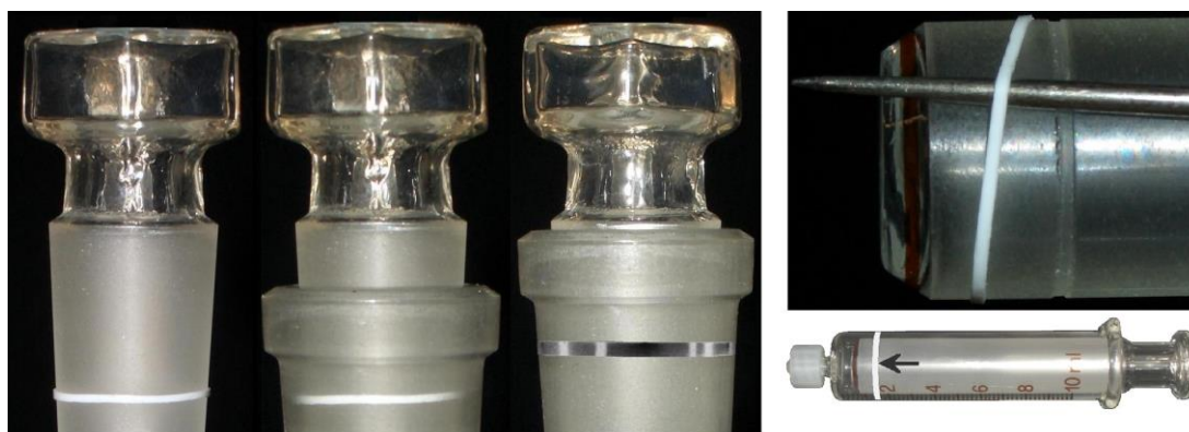
Fig.1. Left: PTFE-sealing ring fixed elastic (no groove necessary). Middle: Sealing ring intransparent without pressure. Right: Sealing ring transparent under sealing pressure. Far right: A similar PTFE ring and a piston groove make an all-glass-syringe gastight.
