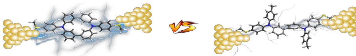
Caption: Cyclic (left) and acyclic (right) bis(triarylamines) shown between two gold electrodes.
